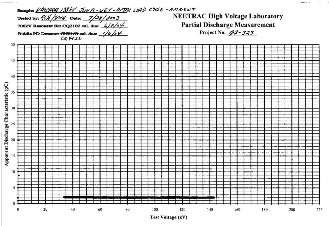
Figure 3 - Partial Discharge Measurement at Ambient after Heat Cycling
