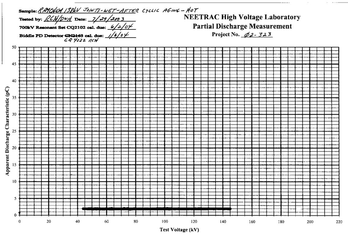
Figure 4 - Partial Discharge Measurement at Elevated Temperature after Heat Cycling
