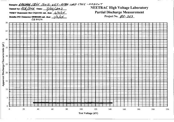
Figure 3 - Partial Discharge Measurement at Ambient after Heat Cycling
