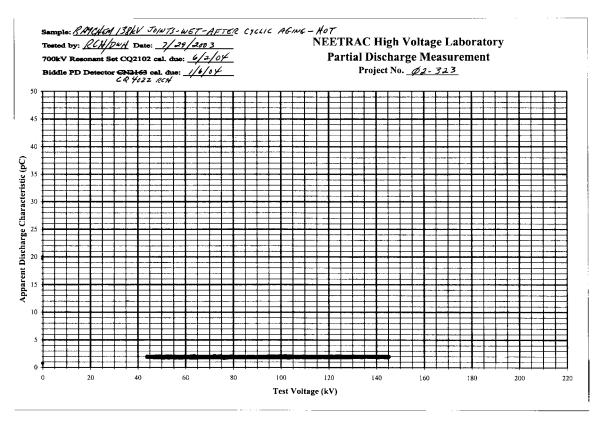
Figure 4 - Partial Discharge Measurement at Elevated Temperature after Heat Cycling
