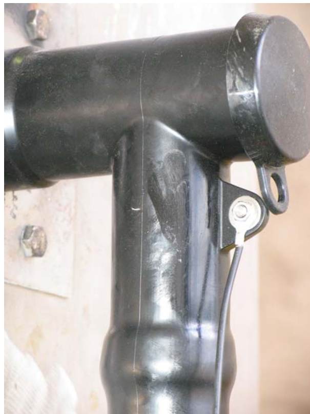
Figure 20: Test object No. 11 before the screen fault current initiation test (unearthed or impedance-earthed systems) point of arc initiation
