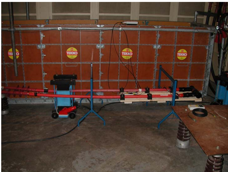
Figure 13: Arrangement for electrical heat cycling test in air for test series D1
