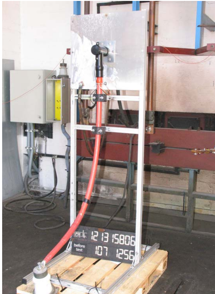
Figure 15: Test object No. 10 before the screen fault current initiation test (solidly earthed systems)
