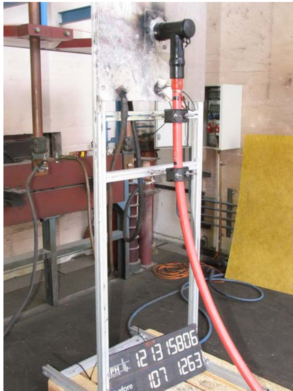
Figure 19: Test object No. 11 before the screen fault current initiation test (unearthed or impedance-earthed systems)
