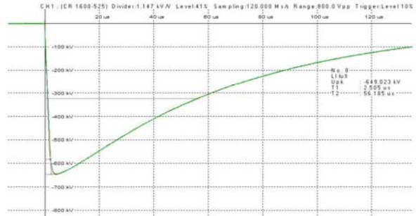
No. 8 LI full Upk: -649.023 kV T1: 2.505 us T2: 56.185 us
